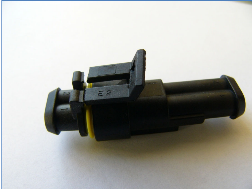
Connecting test after refrigerating connector down to -15C
